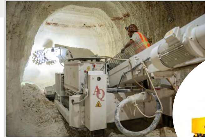
Roadheader tunneling machine
