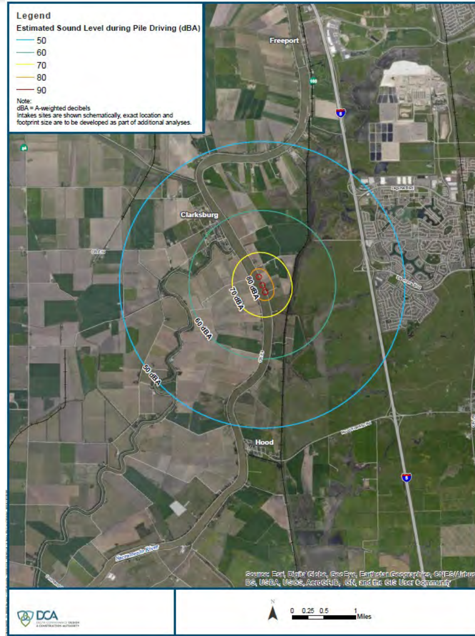
Typical Pile Driving Noise Without Noise Reduction Equipment
