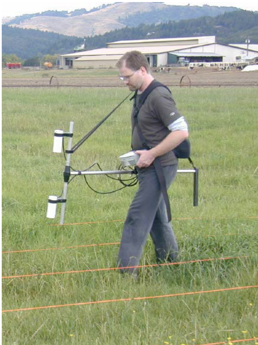
Figure 1. Cesium Vaper Total Field Magnetometer. Source: Rogers et al. 2005
