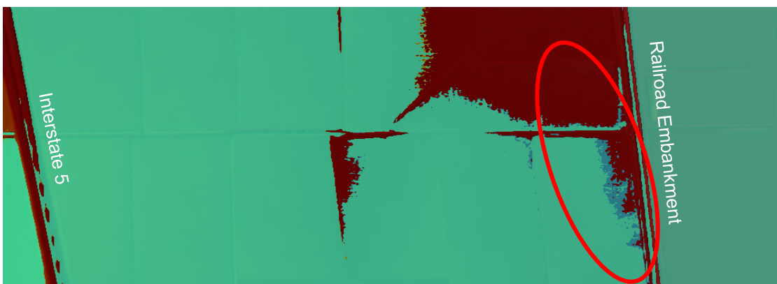
Figure A3-16. 100-year Floodplain under Existing Conditions and Hydraulic Model Scenario 2 north of Twin Cities Complex Site
