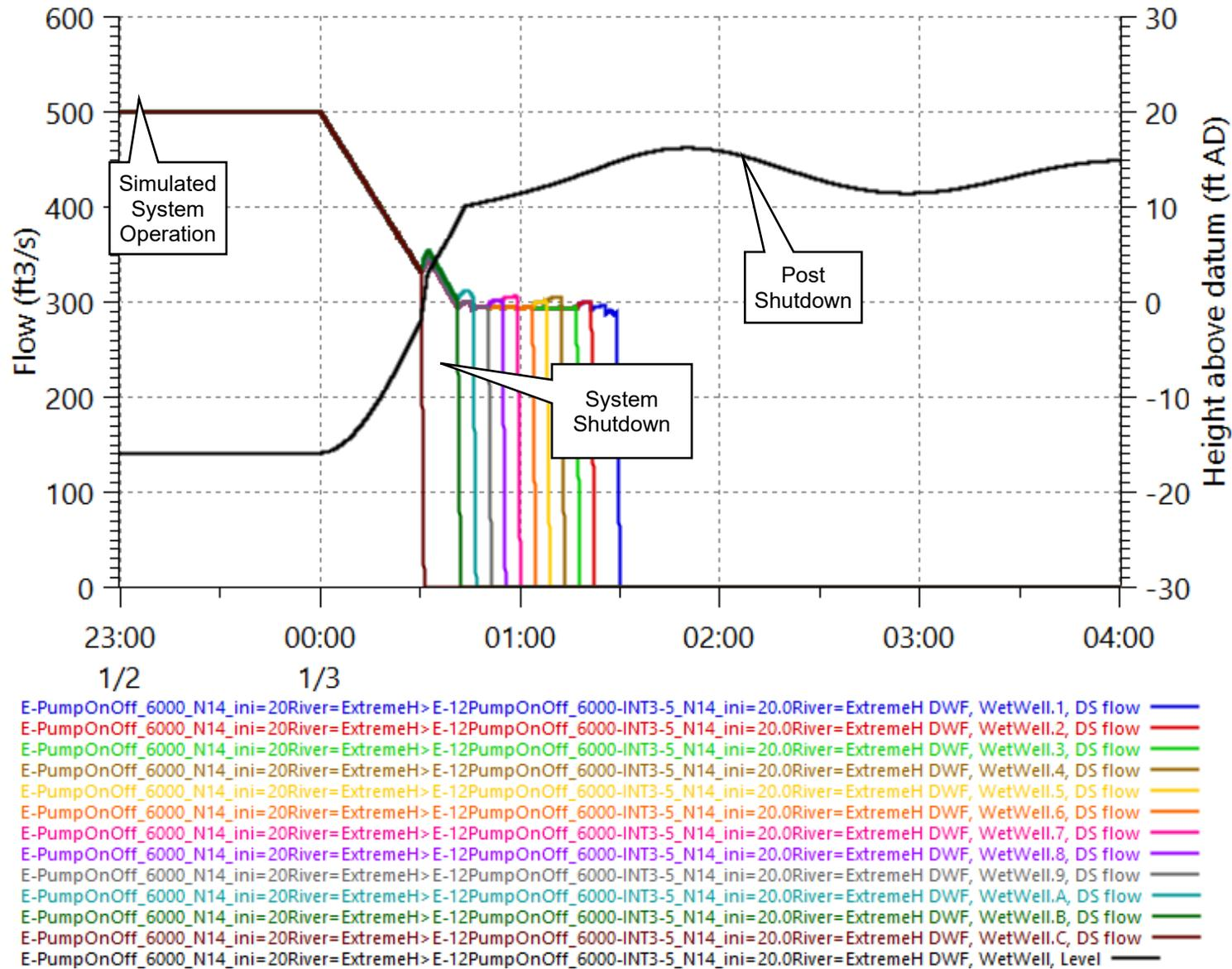
Figure 14. Pump Shut Down and Wet Well Water Level, 6000 cfs, High River, Manning's n= 0.014
