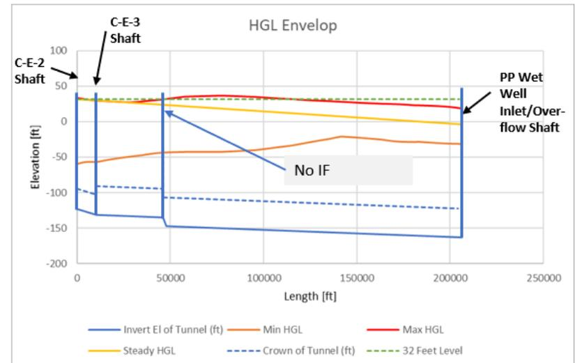
Figure 7. Condition 2, Maximum and Minimum Hydraulic Grade Lines
