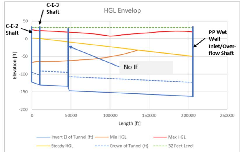
**Figure 8. Condition 3, Maximum and Minimum Hydraulic Grade Lines**
