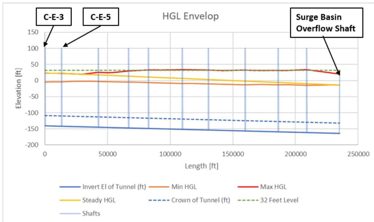
**Figure 45. Scenario 2 – Bethany Reservoir Alignment Main Tunnel; Project Design Capacity 6,000 cfs; High River Level; Minimum and Maximum Hydraulic Gradeline Profiles**
