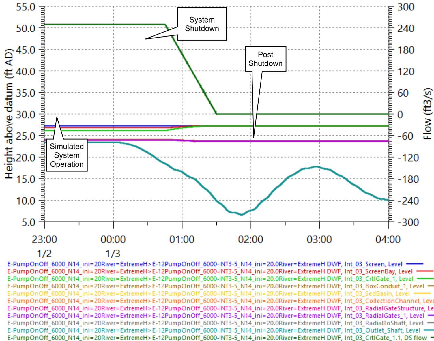
Figure 34. C-E-3 Flow and Water Levels during System Shut Down, High River, Manning's n= 0.014
