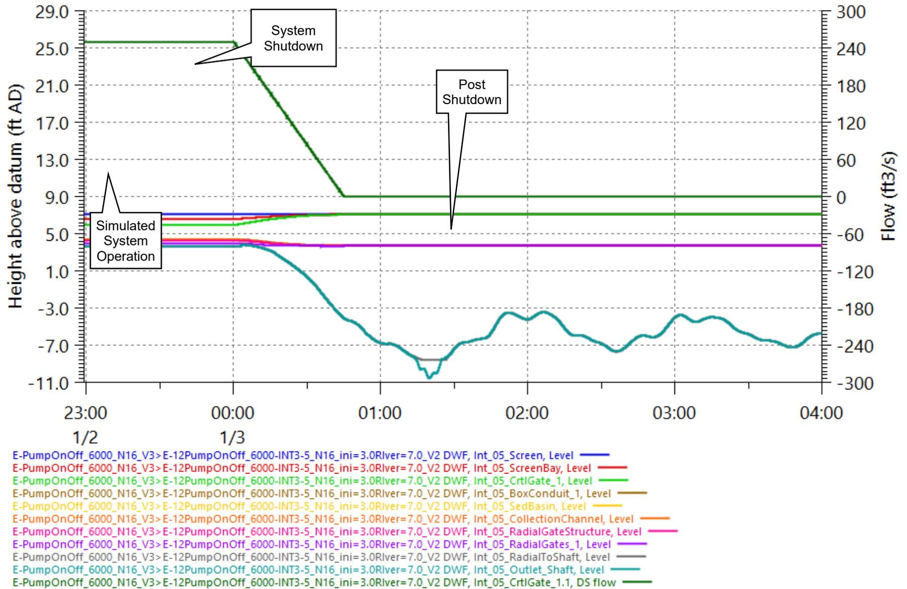
Figure 35. C-E-5 Flow and Water Levels during System Shut Down, Low River, Manning's n= 0.016
