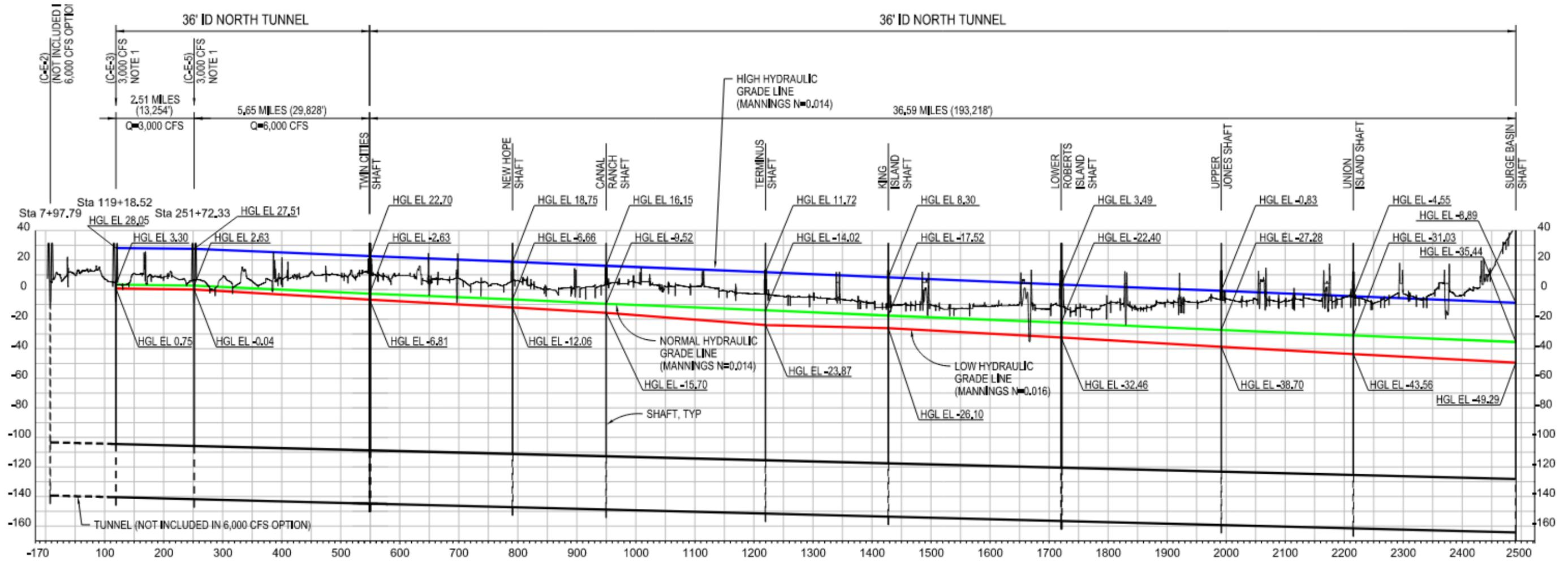
Figure 42. Steady-state HGL; 36-foot-diameter Tunnel; 6,000-cfs Project Design Capacity – Low, Normal, High River Levels
