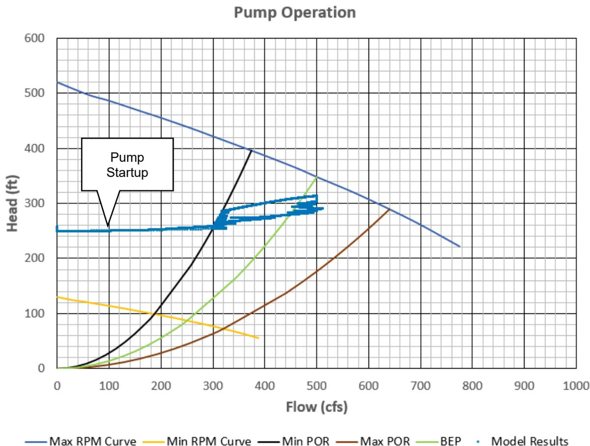
Figure 2. Example RTC Pump Operation Scatter Plot
