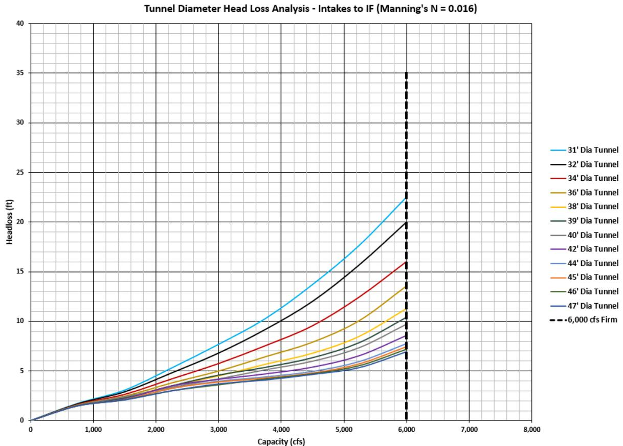
Figure 2. Flow Capacity versus Head Loss for Candidate Tunnel Diameters up to Maximum Design Flow 6,000 cfs
