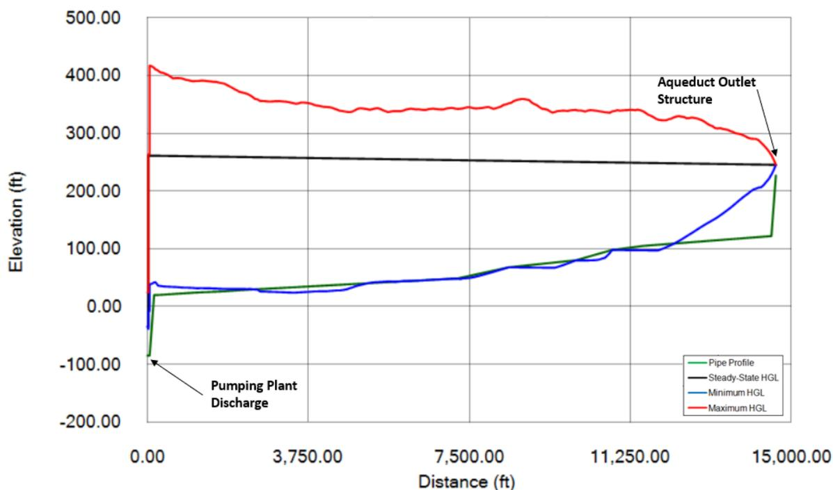
**Figure 46. Bethany Reservoir Aqueduct; Design Capacity 1,500 cfs; Minimum and Maximum Hydraulic Gradeline Profiles**
