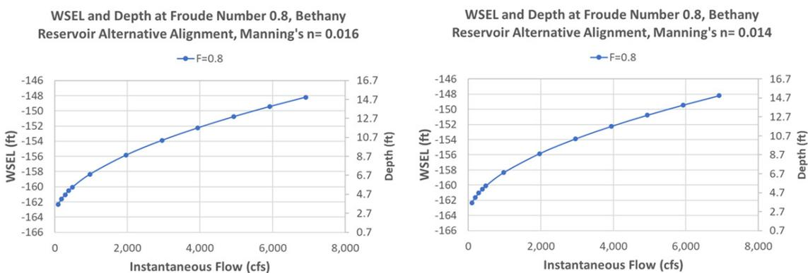
**Figure 48. Instantaneous Flow and Level at Froude Numbers of 0.80, 0.85, 0.90, and 0.95 (Left: Manning’s  $n = 0.016$ , Right: Manning’s  $n = 0.014$ )**
