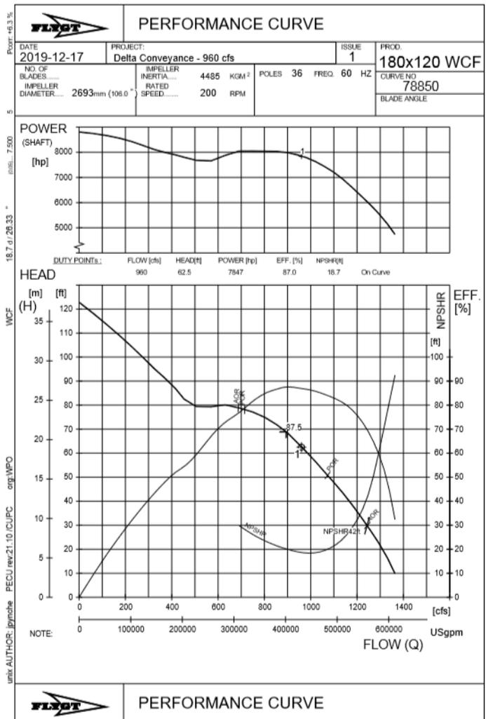
**Figure 5. Flygt Pumps’ Characteristic Pump Performance Curve, Model 180x120 WCF**
