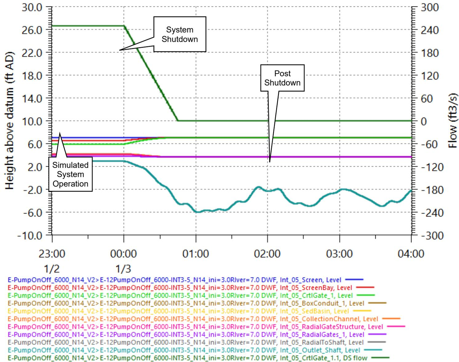
Figure 37. C-E-5 Flow and Water Levels during System Shut Down, Low River, Manning's n= 0.014
