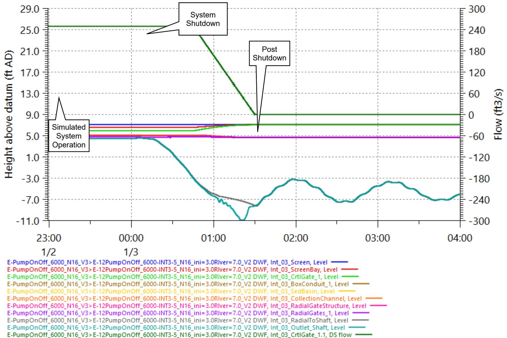
Figure 31. C-E-3 Flow and Water Levels during System Shut Down, Low River, Manning's n= 0.016
