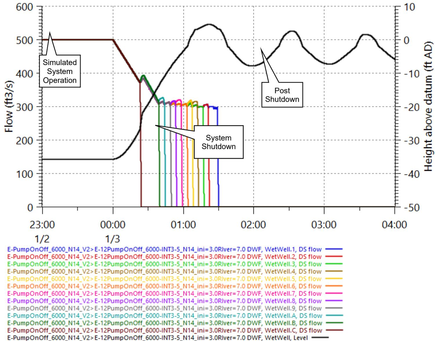
Figure 13. Pump Shut Down and Wet Well Water Level, 6000 cfs, Low River, Manning's n = 0.014
