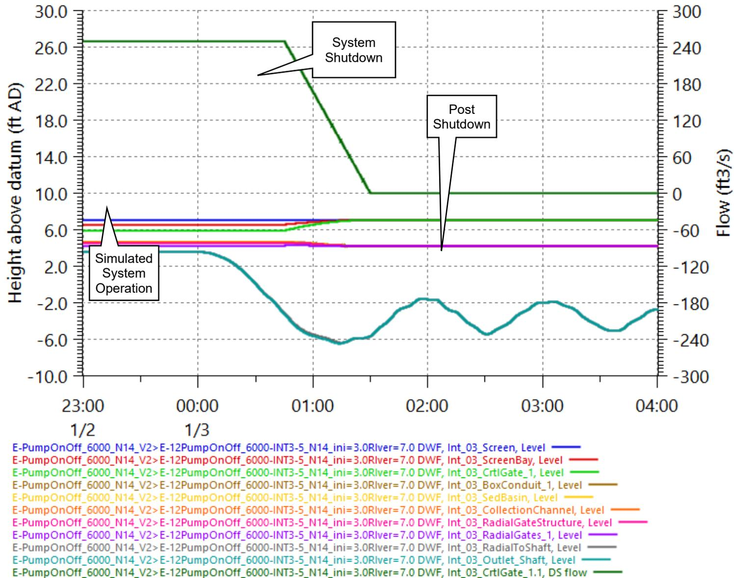
Figure 33. C-E-3 Flow and Water Levels during System Shut Down, Low River, Manning's n = 0.014
