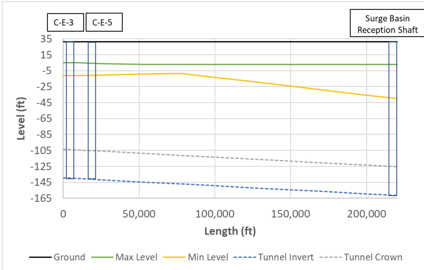
Figure 40. Minimum and Maximum WSEL Profile Startup and Shutdown Scenario, Bethany Reservoir Alignment, 6000 cfs, Manning's  $n$  0.016, Low River
