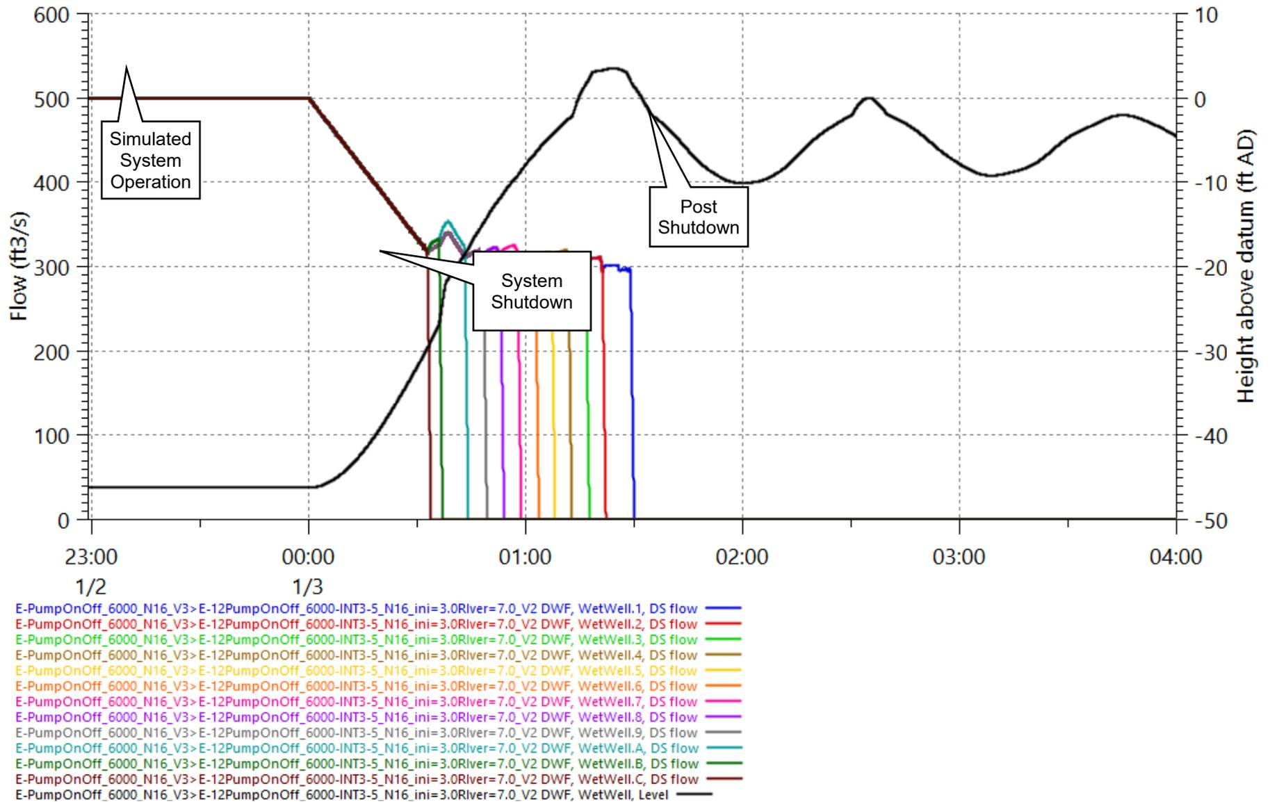
Figure 11. Pump Shut Down and Wet Well Water Level, 6000 cfs, Low River, Manning's n = 0.016
