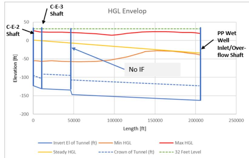
**Figure 6. Condition 1, Maximum and Minimum Hydraulic Grade Lines**
