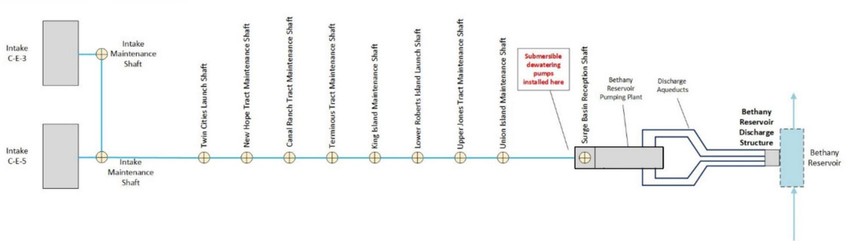
Figure 47. Project Schematic with Proposed Submersible Dewatering Pumps Location
