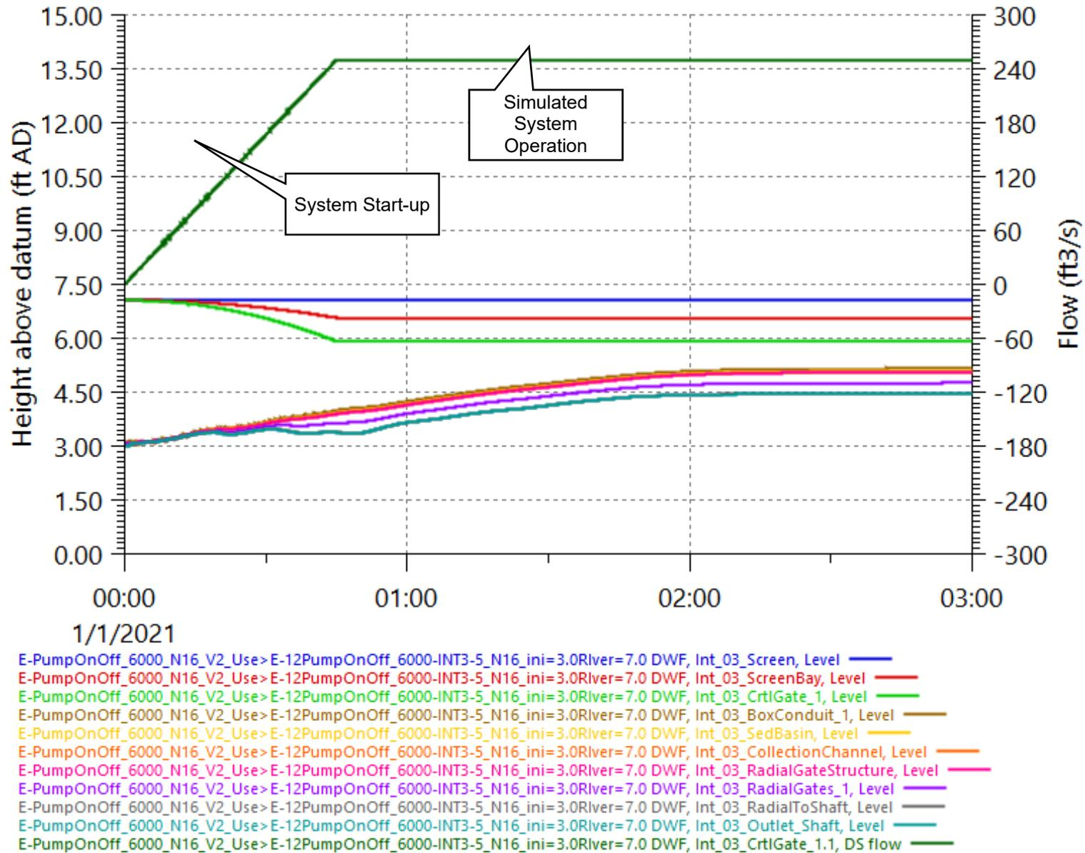
Figure 23. C-E-3 Flow and Water Levels during System Startup, Low River, Manning's n= 0.016
