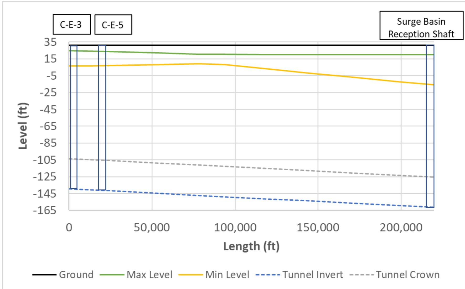
Figure 39. Minimum and Maximum WSEL Profile Startup and Shutdown Scenario, Bethany Reservoir Alignment, 6000 cfs, Manning's  $n$  0.014, High River level
