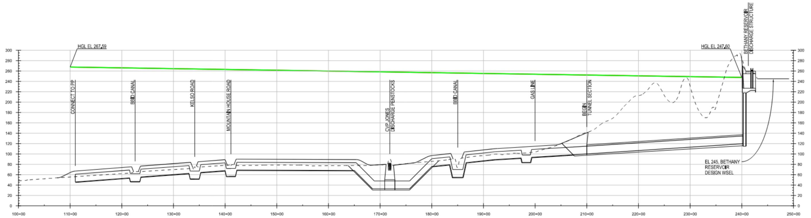
Figure 43. Maximum Steady-state HGL; Bethany Reservoir Aqueduct; 1,500 cfs
