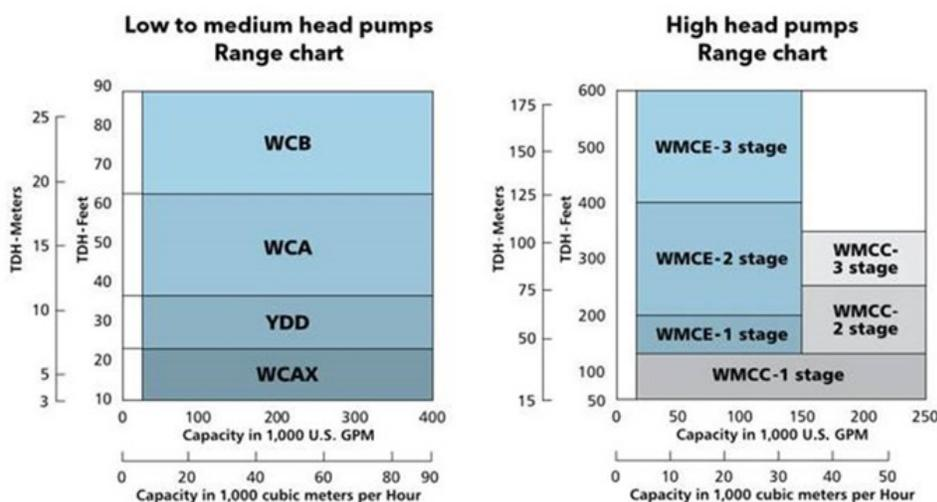
Figure 4. Low to High Head Range Chart for Flygt Large Vertical Column Pull-Out-Style Pumps
