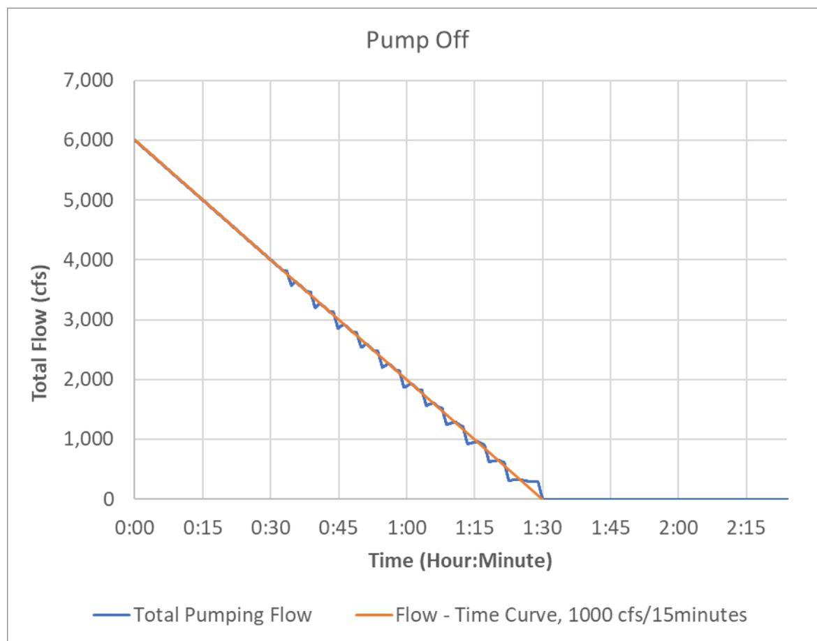
**Figure 6. Real-time Control on Pump Shutdown Operation**
