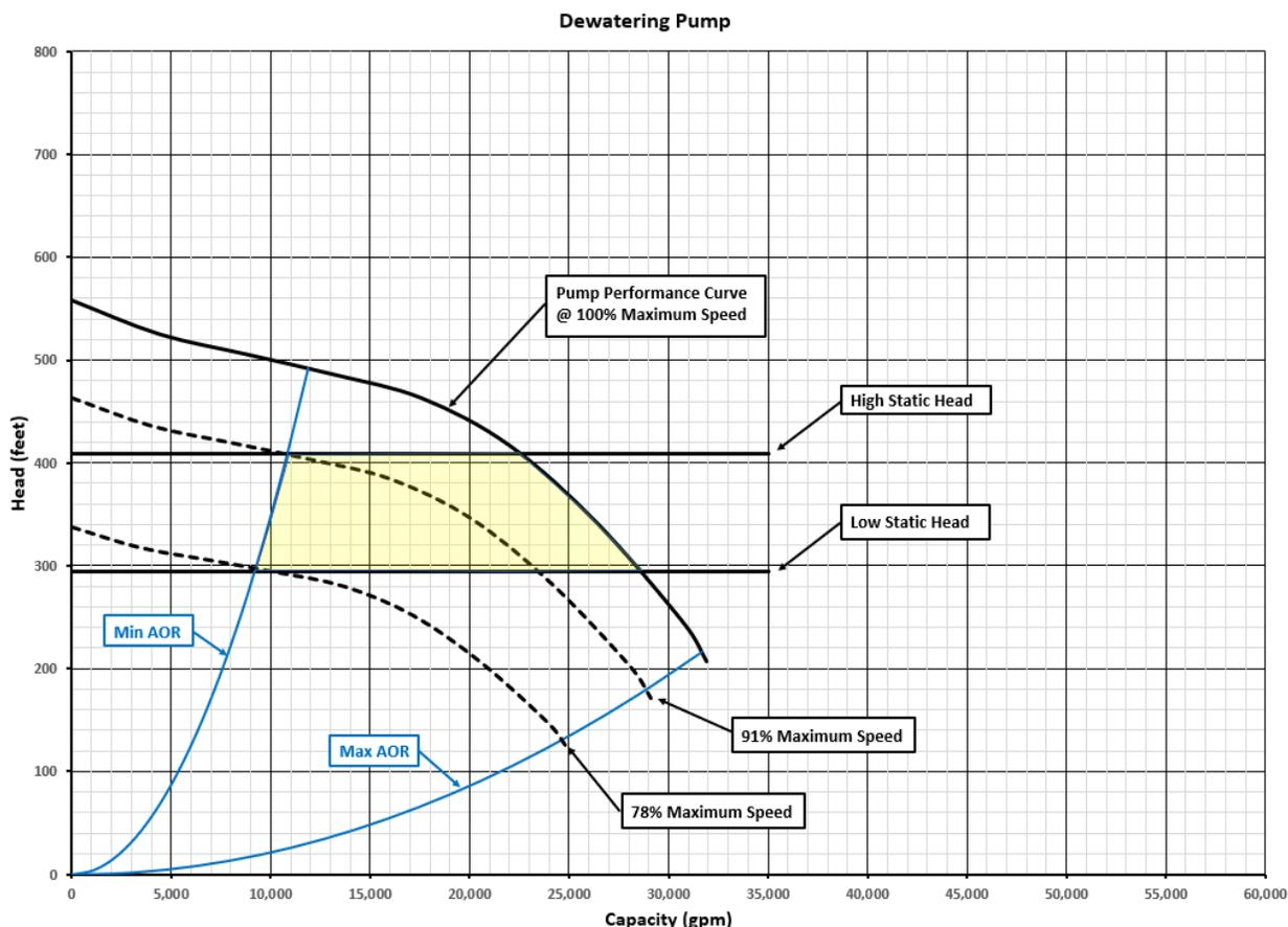
**Figure 49. Candidate Pump Performance Curve Versus System Head Curves**
