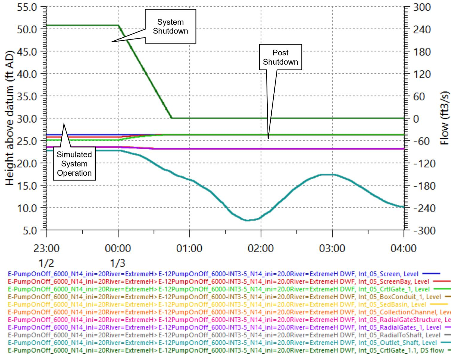
Figure 38. C-E-5 Flow and Water Levels during System Shut Down, High River, Manning's n= 0.014
