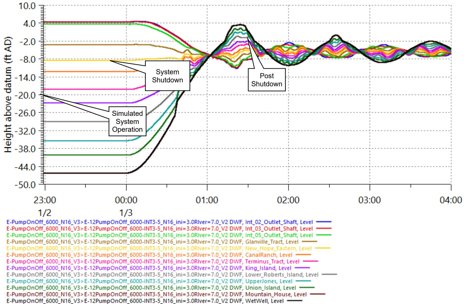
Figure 19. Tunnel Shaft Water Levels during System Shut Down, 6000 cfs, Low River, Manning's n= 0.016
