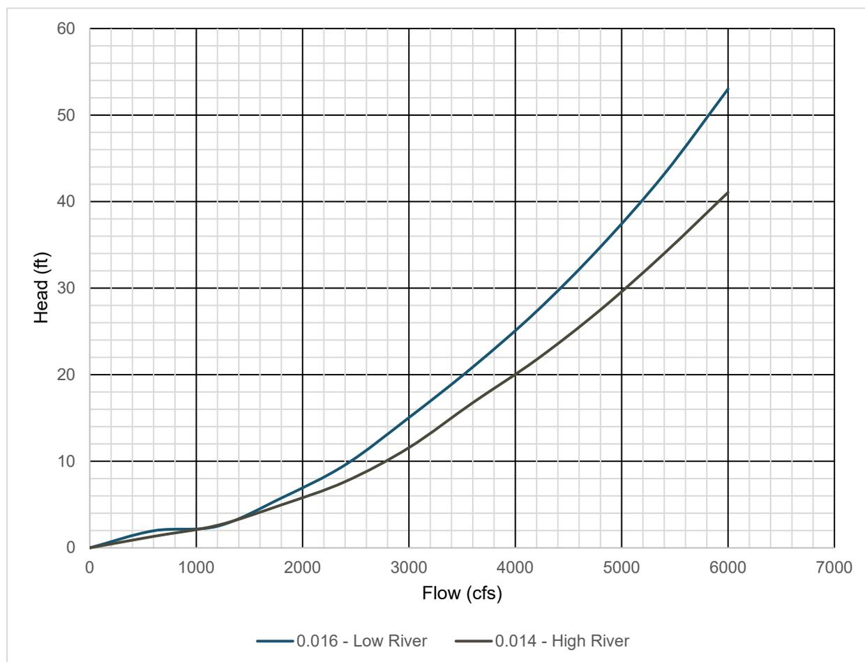
**Figure 41. System Head Curves – 36-foot-inside-diameter Tunnel with a Project Design Capacity of 6,000 cfs**
