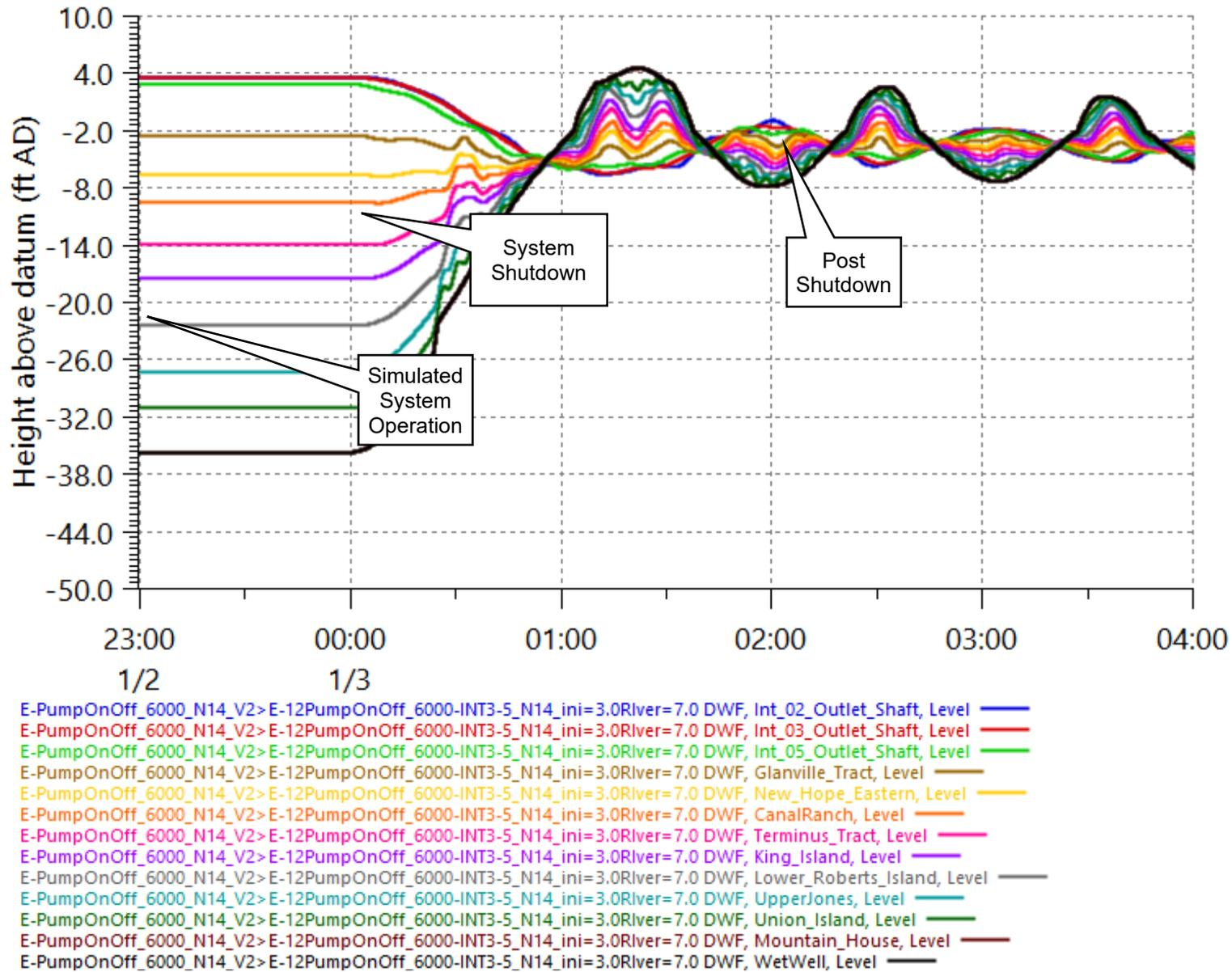
Figure 21. Tunnel Shaft Water Levels during System Shut Down, 6000 cfs, Low River, Manning's n= 0.014
