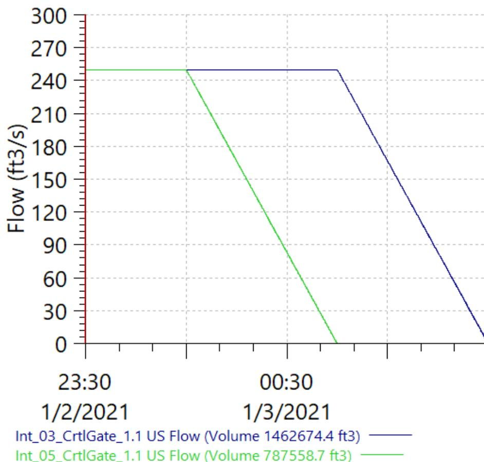
**Figure 5. Intake Control Gate Shutdown Operation**
