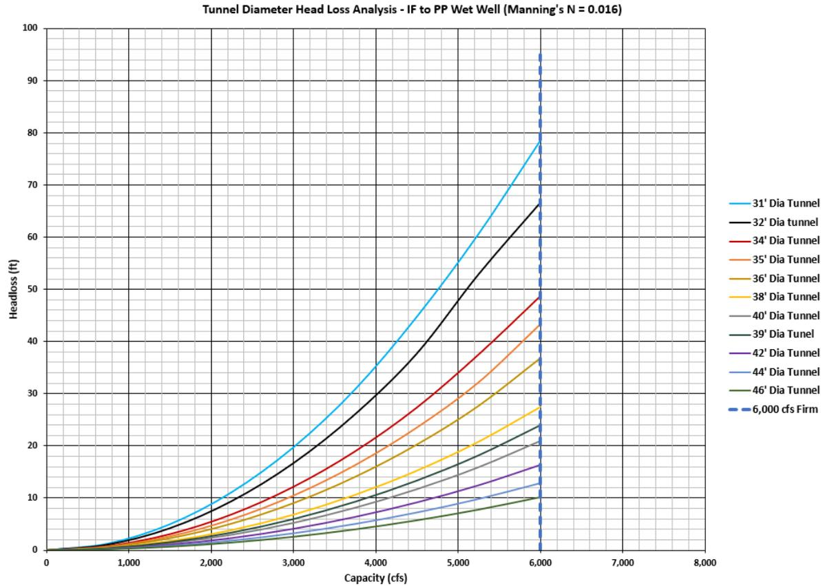
Figure 3. Flow Capacity versus Head Loss for Candidate Tunnel Diameters up to Maximum Design Flow 6,000 cfs
