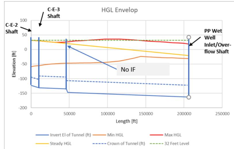
**Figure 9. Condition 4, Maximum and Minimum Hydraulic Grade Lines**
