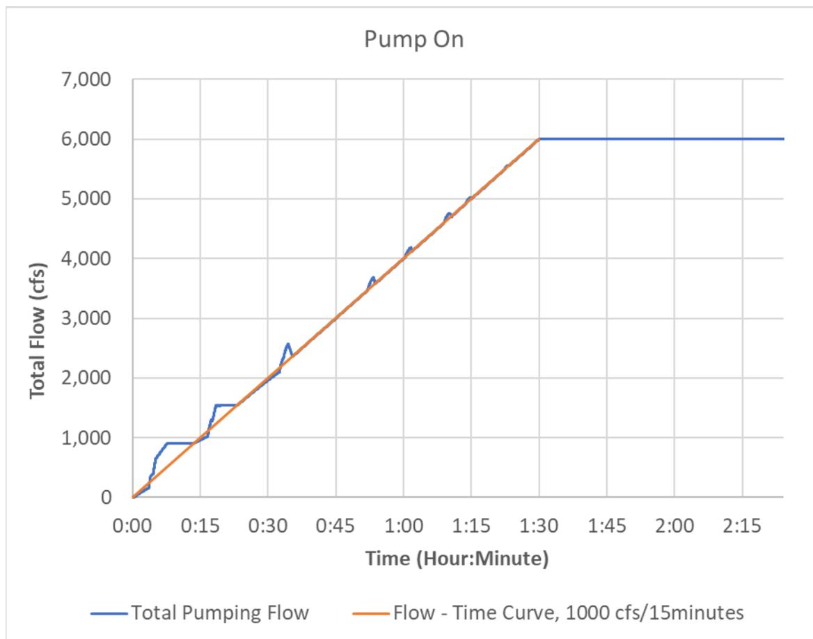
**Figure 4. Real-time Control on Pump Startup Operation**
