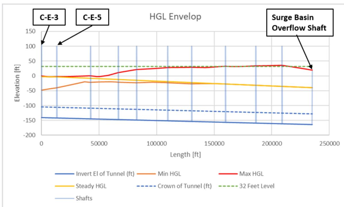
Figure 44. Scenario 1 – Bethany Reservoir Alignment Main Tunnel; Project Design Capacity 6,000 cfs; Low River Level; Minimum and Maximum Hydraulic Gradeline Profiles
